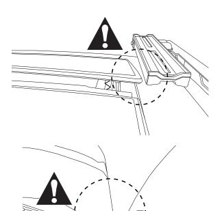
When opening rear door, ensure vehicle door does not come into contact with platform.
